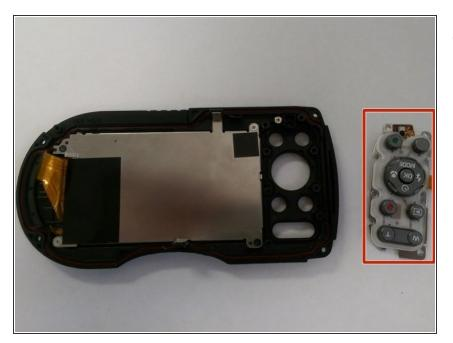
Disconnect the flex cables and replace the menu pad button or button component.
