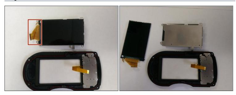
• Detach flex cable and replace screen component.
