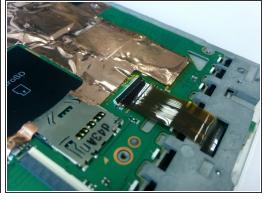
Carefully unplug buses. For the screen bus. Simple pull it from connector. For the hard keys bus.
