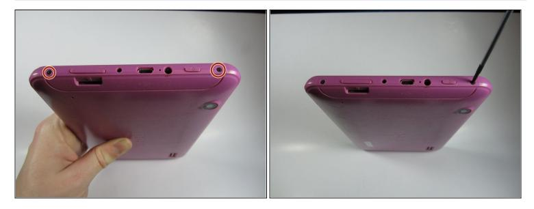
• Use a Phillips #00 screwdriver to remove both 4.1 mm screws at the top of the device which hold it together.
