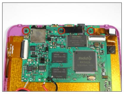
Use a philips #00 screwdriver to unscrew the three 4.064mm screws which attach the motherboard to the front of the device.
