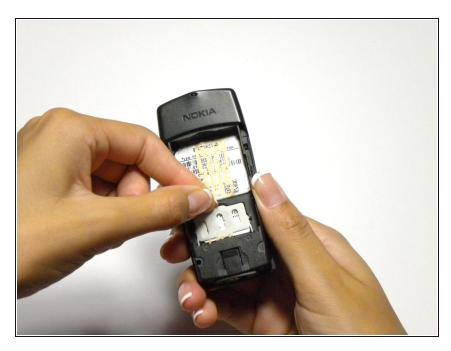
Open the small door covering The SIM card by pulling down from the top
