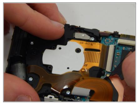
Peel back both the copper sheet and the black tape underneath the panel to expose the connection port.
