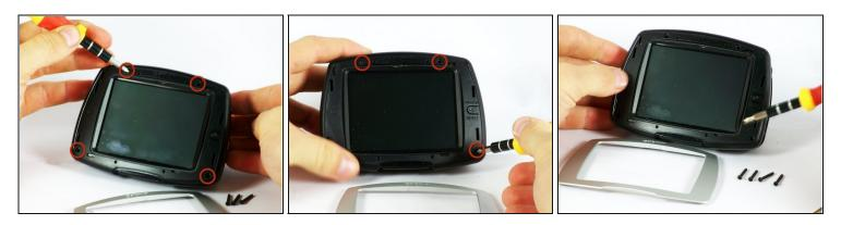
Use a Phillips #00 screwdriver to remove the four screws around the screen.
