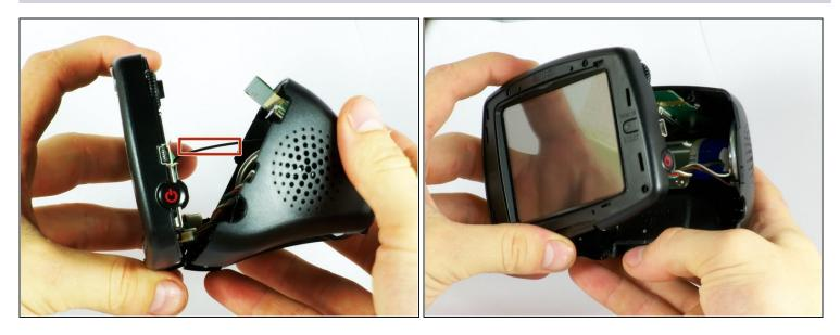
• Gently pull from both ends of the casing to separate the front and back panels.
