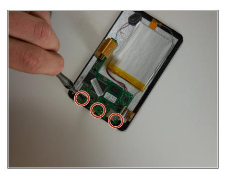
Using the PH#00 screwdriver, remove the three 0.145 inch circuit board screws.
