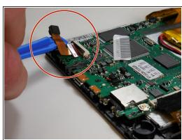
• Lift the hinges on the three ribbon connector clips and disconnect the ribbon connector.
