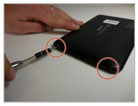
Using the PH#00 screwdriver, remove the two 0.145 inch Phillips head screws.
