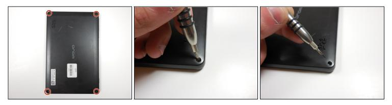
Remove the four 4.8mm mounting screws using a PH00 screwdriver.
