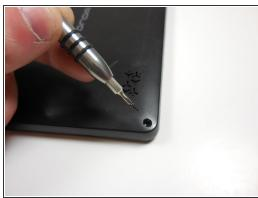
Remove the four 4.8mm mounting screws using a PH00 screwdriver.
