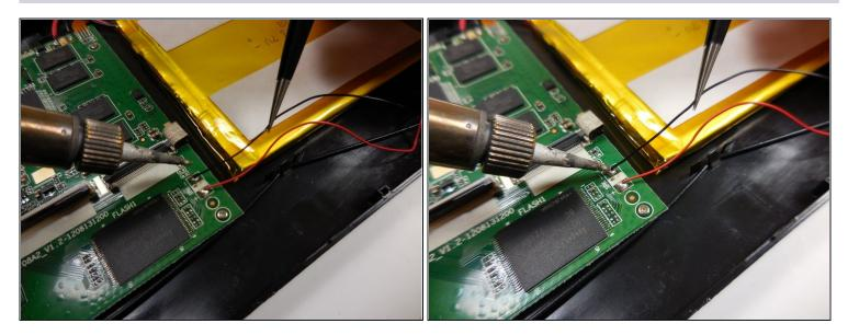
• Desolder the black(-) and red(+) wires connecting the speaker to the motherboard using a soldering iron and <u>tweezers</u> to hold the wire.
