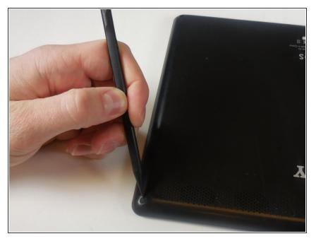
Use a spudger to remove the four rubber screw covers from the four back corners of the tablet.
