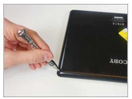
• Place the PH00 screwdriver and use it to remove the four 0.5 cm screws from each corner of the tablet.
