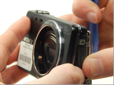
Use the plastic opening tool to gently remove the front and back plates of the camera.
