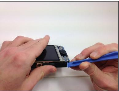
Use a plastic opening tool to gently release the two indicated tabs.
