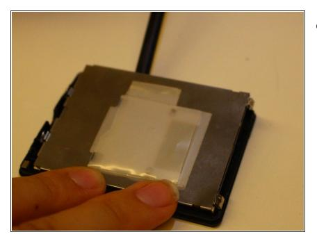
Using a spudger, remove the external shell of the LCD screen leaving only the metal internal circuit board and screen attached.
