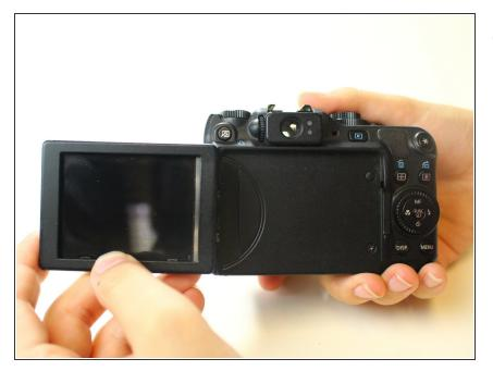
Open the LCD screen from its locked position so the screen is visible.
