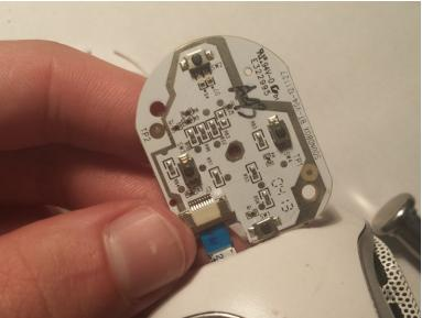
• Using a size 1 PH screw driver, unscrew the two 3.3mm screws holding the cap on.
