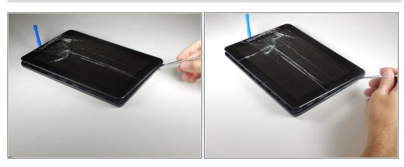
• Slide the metal spudger around the casing to separate it from the inside of the tablet.
