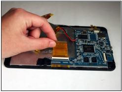
• Once battery is removed, flip up the black lever of the connector that is holding the wide ribbon in place for the screen. Remove the ribbon from the connector.
