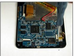
• Rotate the tablet 90 degrees and remove the three (3) 1.3 mm Phillips #00 screws that hold the motherboard in place.
