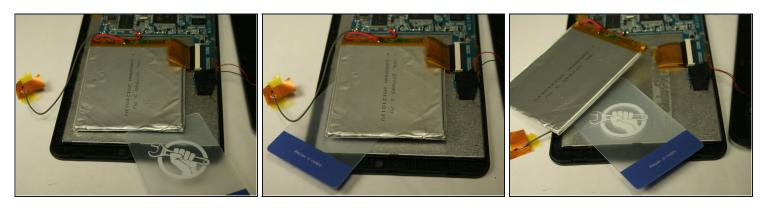
Using a plastic card, gently break the adhesive that holds the battery to the metal screen plate.
