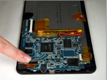
• Lift up the black lever of the connector that holds the camera ribbon in place.
