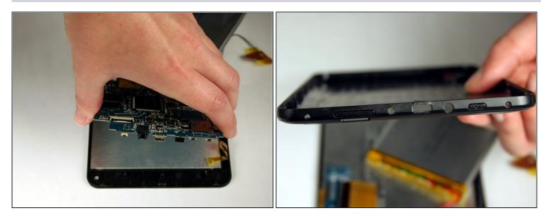
• With the motherboard detached from the screen plate, there is now access to the electrical components under the motherboard and the mechanical button components on the back plate.
