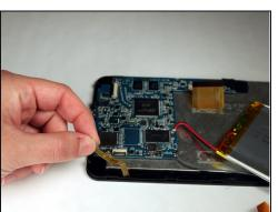
• Rotate the tablet 180 degrees and flip up the black lever of the connector holding the small, yellow ribbon. Remove ribbon from the connector.
