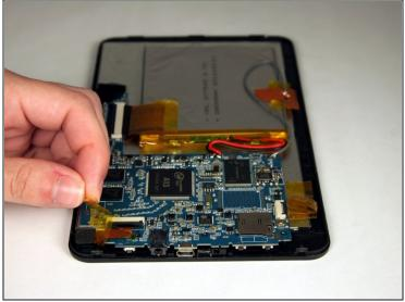
Once the panels are separated, remove the tape holding down the ribbon connector that is connecting the camera to the motherboard.
