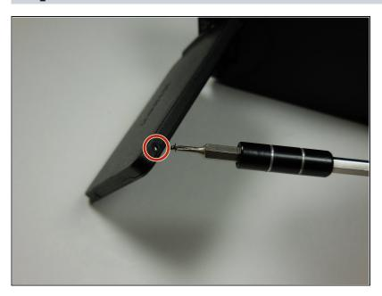
Use a Phillips #00 screwdriver to remove the 4.3 screw on both the top and bottom of the screen's casing.
