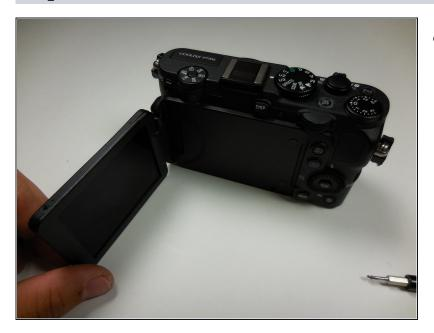
Open the camera LCD screen so it's away from the body of the camera.
