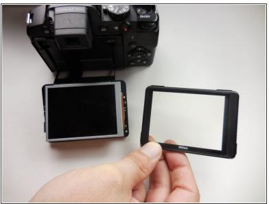
• Use a plastic opening tool to trace around the screen to pop the front and back section apart.
