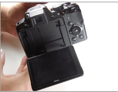
Extend the LCD screen out and turn the camera upside down to get access to the screws on the bottom.
