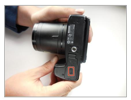
Flip the camera over and push the tab on the battery cover to open the battery compartment.
