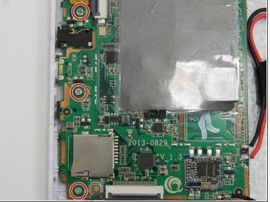
Remove the three 2.5mm screws using the Phillips #00 precision screwdriver that is holding the motherboard in place.
