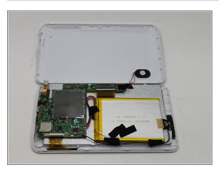
Upon removing the back cover position the tablet as seen in the picture.
