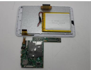
Remove the three wires connected to the battery along with the speaker wires from the motherboard. Then remove the motherboard from the tablet.
