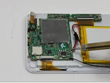
Install the new motherboard by soldering the speaker wires and the battery wires in their intended location. For additional soldering instructions please view this page: <u>How To Solder and Desolder</u> <u>Connections</u> To reassemble your device, follow these instructions in reverse order.
