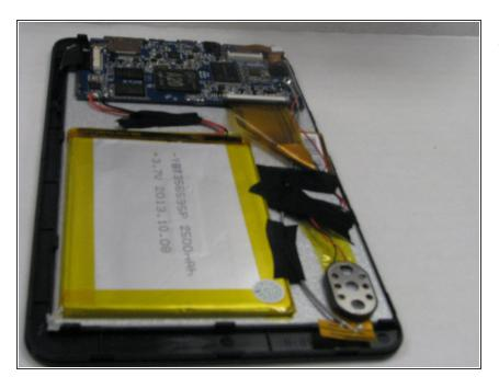
Remove the black tape attaching the wires to the battery.
