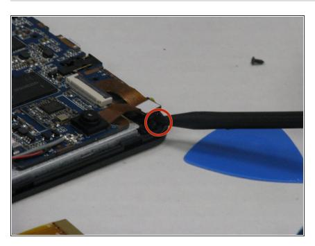
Use the spudger to unhinge the camera from its socket.
