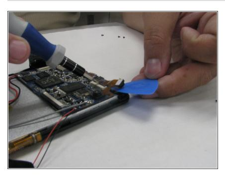
Use the plastic opening pick and the Phillips screwdriver to remove the camera from its soldering on the motherboard, and set it aside to be replaced.
