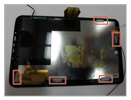
Remove these 2.5mm screws and brackets holding the screen down using a PH00 screwdriver.
