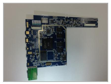
Gently lift the motherboard out of the tablet, make sure no wires are still caught or attached while you lift the motherboard.
