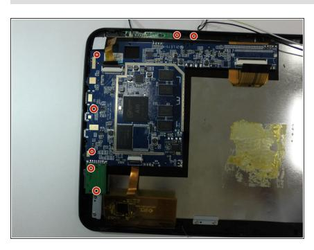
Remove the 3.5mm screws located at these locations shown on the picture by using the PH00 screwdriver.
