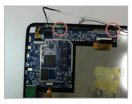
Unsolder these wires from the motherboard, it is a good idea to label these wires as you remove them according to the picture to the left.
