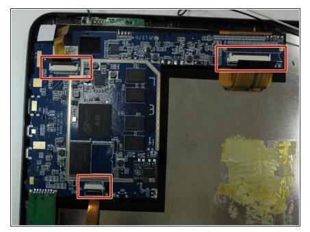
Remove contact strips by lifting gently on the clip indicated in this picture, then pulling strip out of the clip.
