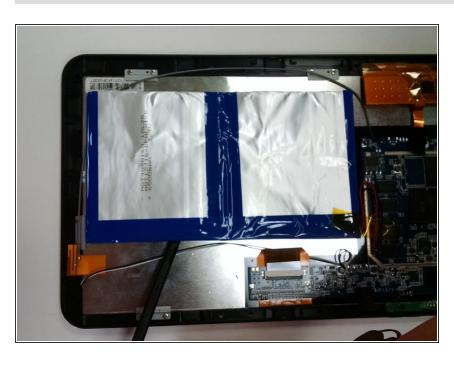
Slide the spudger underneath the battery and gently lift it off of the adhesive.
