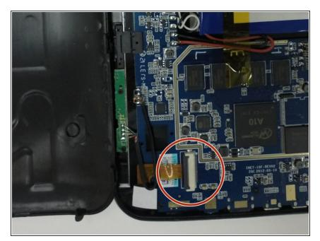
Lift the tab on the wire ribbon shown here
