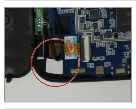
Pull up gently on the camera housing shown on this picture, it is glued in place.
