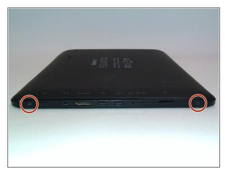
Remove the two 3mm screws using a PH00 screwdriver.
