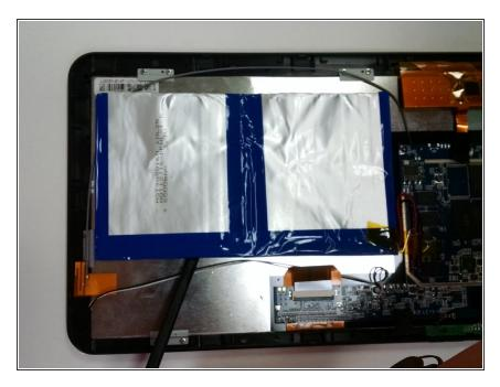
Slide the spudger underneath the battery and gently lift it off of the adhesive.
