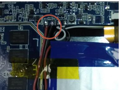
Place the new battery in the same location and connect the wires the same way as the previous battery.
