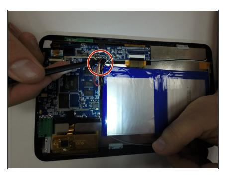
Disconnect the wires that connect the battery to the motherboard using the spudger.
