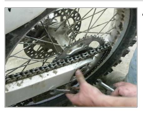
The chain will still be on the sprocket. It is easy to roll it off the side of the sprocket.
