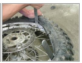
Now do the same method of leverage, but put the tire back on. (Be extremely careful to not pinch the tube between the tire spoon and the rim.)
