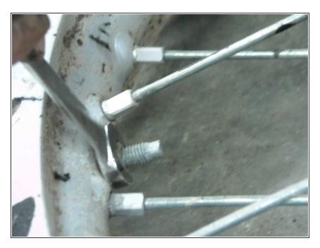
Do not take the nut all the way off of the bead lock, Just make sure it as loose as possible.
