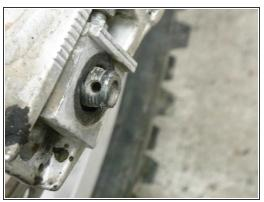
Now the tire is ready to go back on. When putting the tire back on make sure the spacers are in the correct areas. make sure the chain is on the sprocket. Lastly, make sure the break disc is inside the break pads.
