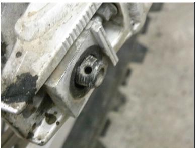
First pull the cotter key out of the axle that holds the tire on. Then pull the nut off of the axle.
