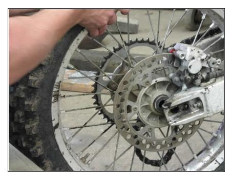
The bolt is off the axle already so use a rubber mallet to beat the axle out of the wheel. After the axle is far enough through, you can pull it out the rest of the way with your hands.
