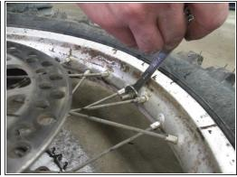
The wheel is now off. Now you should take the valve core out of the tire with a <u>valve core tool</u>, and release all the air. Use a size 12mm wrench and take the nuts off the valve stem, and the bead lock. Which is the other thing in the rim with a nut on it besides the valve stem.
