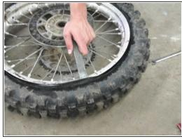
After all the air is gone you need to break the bead loose on both sides. Just push down so the tire goes away from the rim. Then spray soapy water in between the rim and tire all the way around on both side. Then take the tire iron and wedge it between the rim and tire. Once wedged use leverage from the rim to pull the tire up and away.
