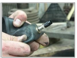
Once the tire is back on the rim add more air this should push the bead lock out. Now you can put the nut back on the bead lock as well.(do not tighten yet.) make sure the tire is at the correct pressure and everything looks good, now you can tighten down the bead lock, and the valve stem. After the valve stem is tight put the second nut on.
