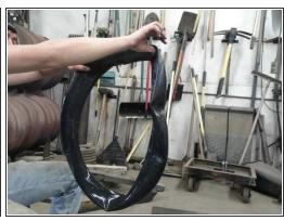
• If you are actually changing the whole tire repeat this to pull the rest off the tire off. If not pull the tube out of the slit that you have made by pulling the half of tire off.
