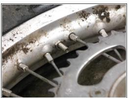
• Put the new tube in the tire. put the valve stem through the hole in the rim then put one of the nuts on it.( not the bead lock.) Add a little bit of air to the tube.(the less you use the better off you are.)
