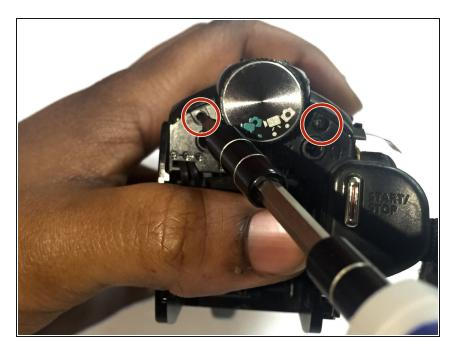
Remove the two 3x4 mm Phillips screws beneath the two covers (AV & DCIN).
