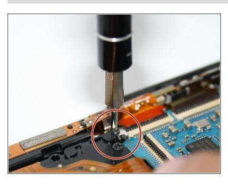
Remove the 4 mm Philip screw located above the center film strip with the Philips screw driver. This will allow the top frame to come loose to take off.
