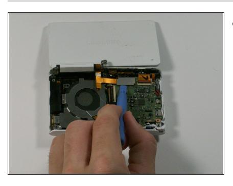
Use plastic opening tool to disconnect screen connector from the control board.
