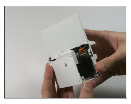
Remove the back casing by just carefully pulling the casing off of the camera.
