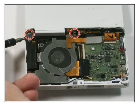
Use the Phillips #00 screw driver to remove the four 2.381 mm screws next to the screen hinge.
