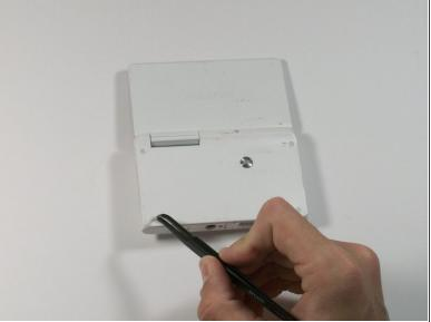
Use tweezers to remove the four rubber screw covers.
