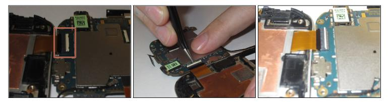
• Remove the gold ribbon cable by lifting tab at the back of the socket, using a spudger or tweezers.
