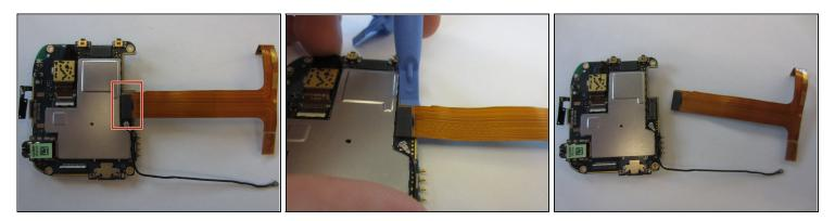
• Noting that the rear side of the black ribbon cable is gold, use a spudger or an opening tool to gently disconnect it from the motherboard by levering it up at the right side
