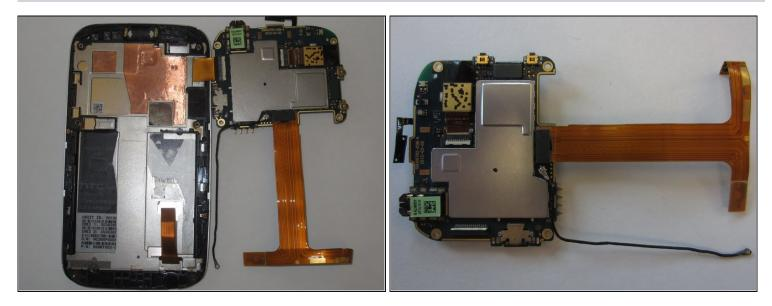
• Gently pull the logic board to the right and it will disconnect from the chassis.
