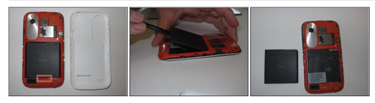
• Lever the battery out from the bottom end first.
