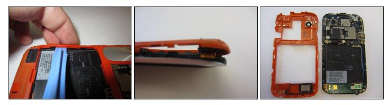
• Use an opening tool or a spudger to gently remove the rear frame.
