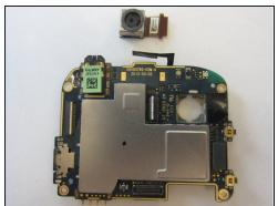
• Preferably using tweezers, gently pull the camera assembly up from the motherboard, and away from the connector and the ribbon cable will slide out easily.
