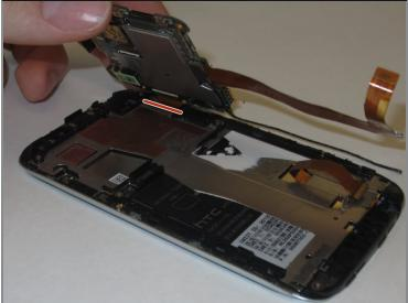
• Gently pry logic board from the casing by lifting the left side up, as if there was a hinge on the right, folding it over the right edge where you will see a gold/orange ribbon cable.
