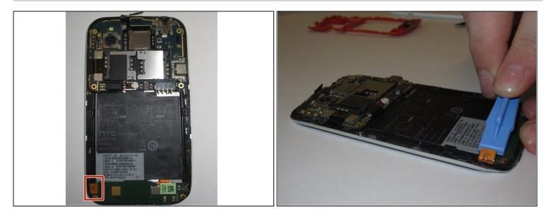
• Remove the connector on left side of the Navigation board by unplugging/prying the orange ribbon.
