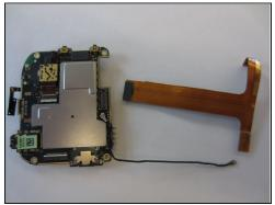
Noting that the rear side of the black ribbon cable is gold, use a spudger or an opening tool to gently disconnect it from the motherboard by levering it up at the right side
