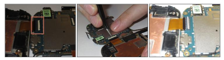
• Remove the gold ribbon cable by lifting tab at the back of the socket, using a spudger or tweezers.
