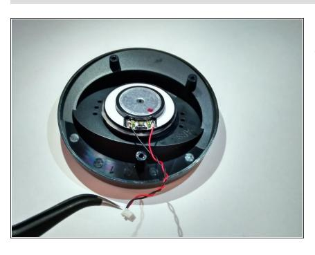
Use super glue to fasten the replacement speaker into the speaker housing. To reassemble your device, follow these instructions in reverse order.
