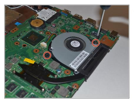
Remove the two 5 mm screws with a Phillips #00 screwdriver.
