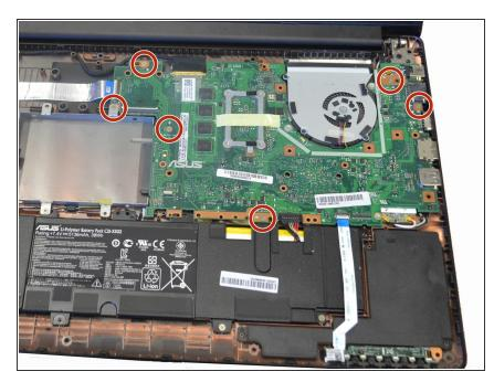
Remove the six 5 mm screws using the Phillips #00 screwdriver.
