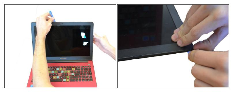
Remove the trim from the monitor by using the Plastic Opening Tool to carefully pop off the clips around the parameter.
