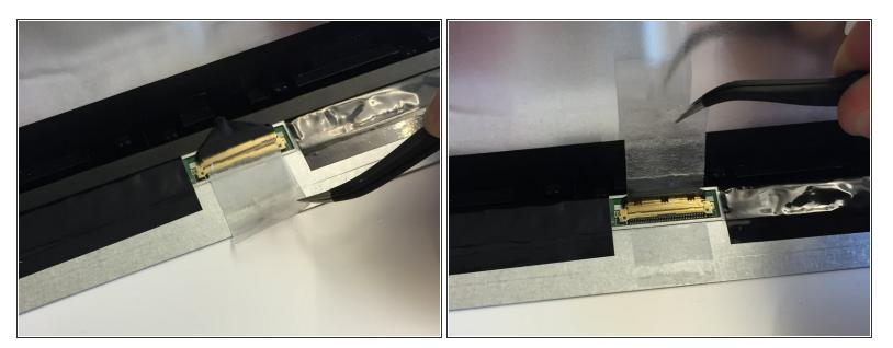
• Peel off the clear tape that is securing the video cable connector using your fingers or tweezers.
