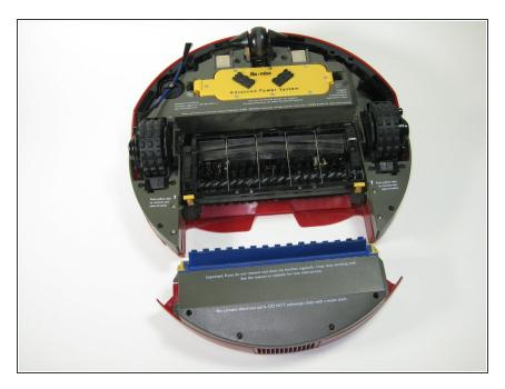
Remove the particle bin from the back of the Roomba.
