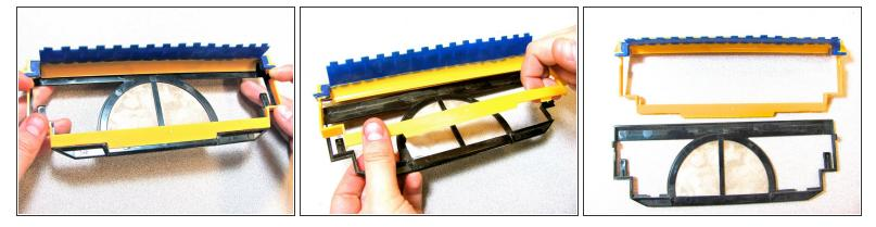
Pinch the black plastic of the filter and pull it away from the yellow filter holder.
