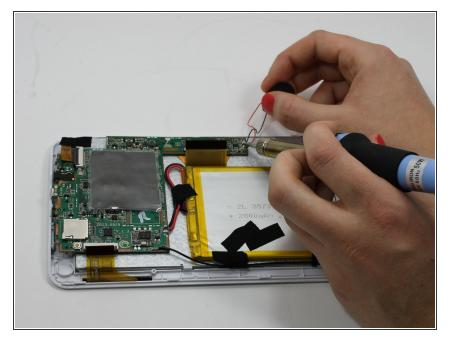
Install the new speaker by soldering the wires to the motherboard. For additional soldering instructions please view this page: <u>How To</u> <u>Solder and Desolder Connections</u>
