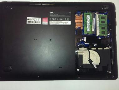
Remove the panel by sliding down and lifting it away from the computer, exposing the RAM and hard drive.
