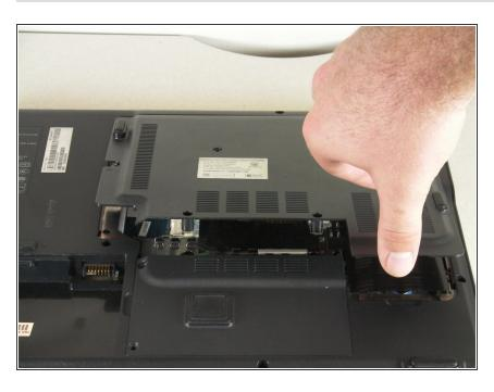
Lift and remove the panel.
