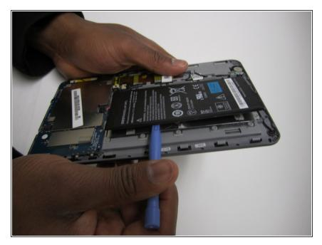
Use the plastic opening tool to lift the battery off of the back panel. The adhesive used is strong so apply force during removal.
