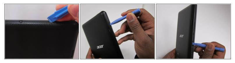
Insert a plastic opening tool into a gap near the charging port at the top of the device. Slide the tool
