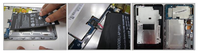
• Lift the battery off of the panel gently. This will disconnect the battery connector from the motherboard.
