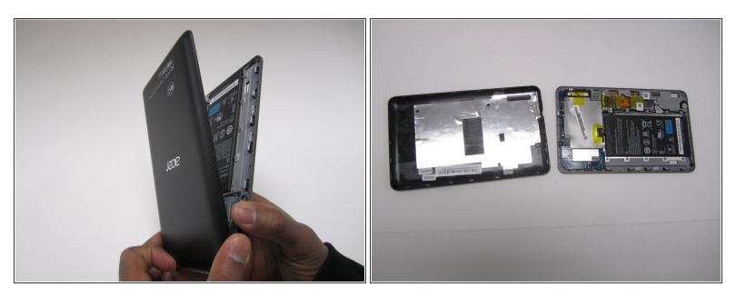
Once all the sides have been separated, you should be able to simply lift the cover off of the device.
