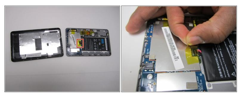
Peel back the plastic tape covering the battery connector.
