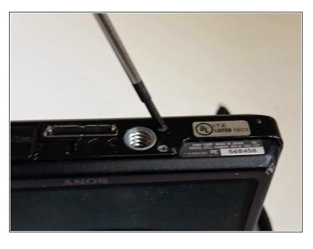
Use the Phillips #00 screwdriver to remove the 4mm length screws.
