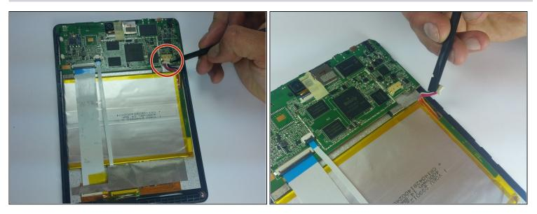
• Use a spudger to carefully disconnect the battery connector from the motherboard.
