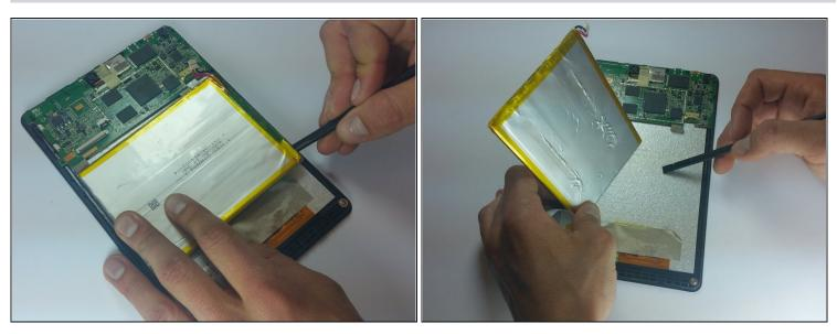
• Using the flat end of a spudger, carefully work the spudger under the battery, lifting it off of the device.
