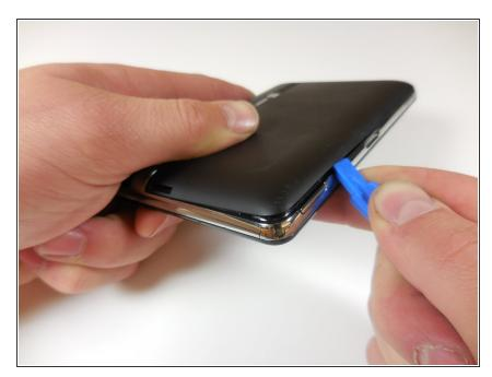
Use the plastic opening tool to separate the tabs on the black back cover of the device by leveraging the tool against the frame around the perimeter of the device.
