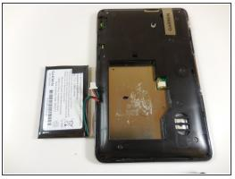
• Use the plastic spudger to lift the battery up and away from the device.
