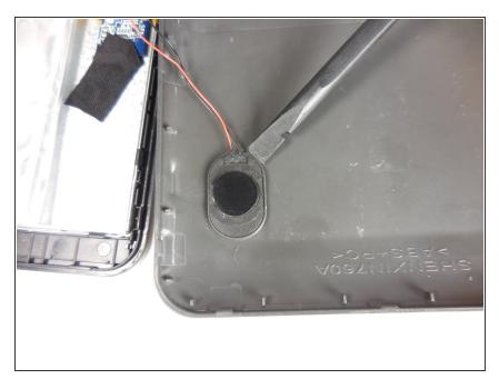
Disconnect speaker (which is attached by black and red wires) from back piece using plastic spudger.
