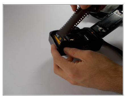
• Place the roll part of the film in the corresponding side.
