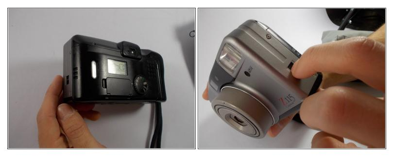
• On the side of your camera, push the strip of black plastic located in between "open" and a down arrow, down to open the camera. The back of the camera will pop open showing the film.
