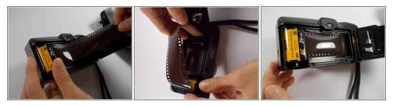
Take the film and feed it through the right side of the plastic cylinder. The film should wrap around it.
