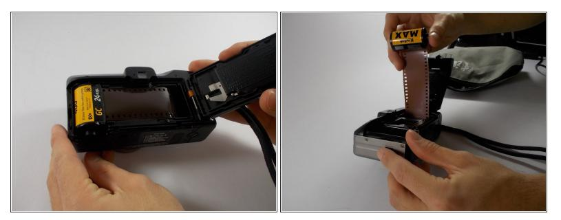
• Locate the side of the film that holds all the film. Push it forward and lift it out of the camera.
