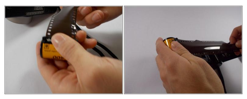
• Take you new roll of film and pull film out until it's the horizontal length of the camera.
