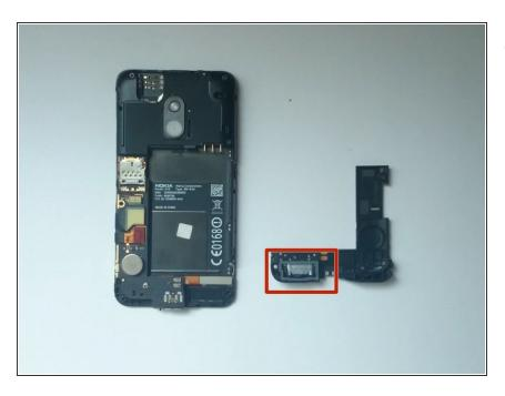
The Loudspeaker is on the lower back cover.
