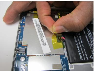
Peel back the plastic tape covering the battery connector.
