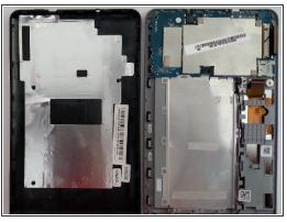
Lift the battery off of the panel gently. This will disconnect the battery connector from the motherboard.
