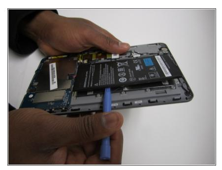
Use the plastic opening tool to lift the battery off of the back panel.
