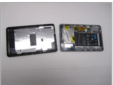
Once all the sides have been separated, you should be able to simply lift the cover off of the device.
