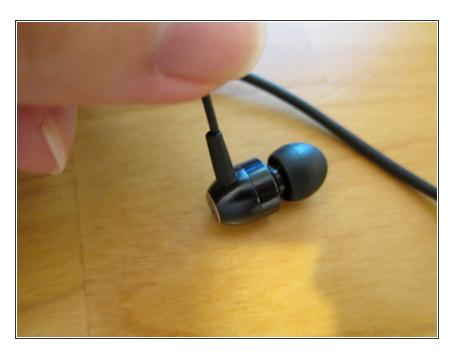
Over time, the plastic grommet that fits between the wire and the hole in the earbud will fall out. This can be caused by pulling on the wire & grommet when removing the earbud from an ear rather than tugging on the earbud's body.
