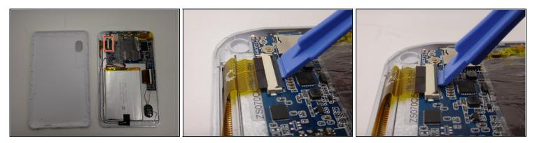
Use the plastic opening tool to gently lift the release lever for the ZIF cable.
