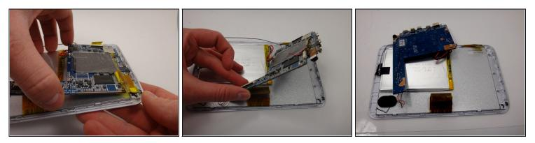
• Remove the motherboard from the casing, being careful not to damage the remaining wires.
