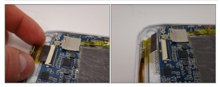
• Gently remove the ZIF cable from the connector.
