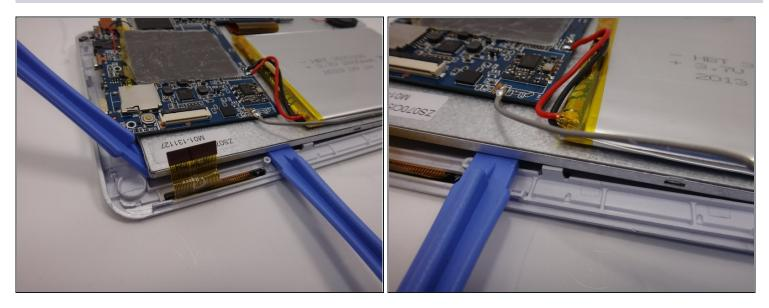
• Using a second plastic opening tool, pry the adjacent side of the metal backing from the front casing/touch screen.
