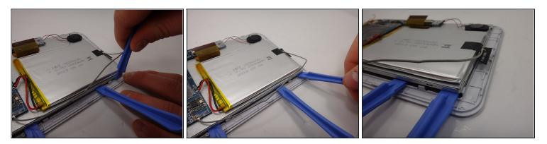
• Use a third plastic opening tool to pry at the corner of the tablet and pop off the metal backing.
