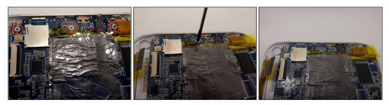
• Remove the three 4mm Phillips #00 screws securing the motherboard in place.
