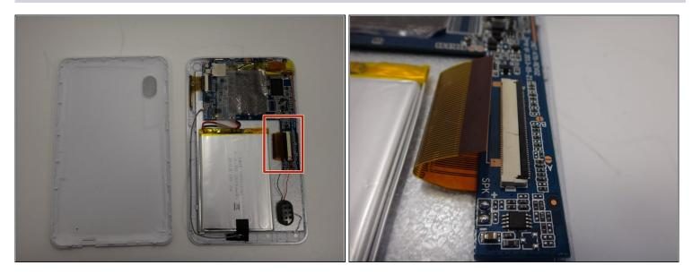
• Disconnect the second ZIF connector using the same method detailed earlier.
