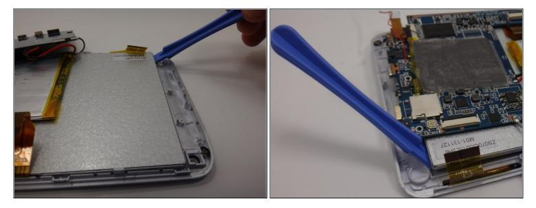
• Starting at the edge, use a plastic opening tool to carefully pry the front casing off of the metal backing.
