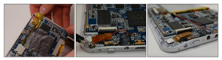
• Locate the microphone. It is at the top of the device and next to the audio jack.
