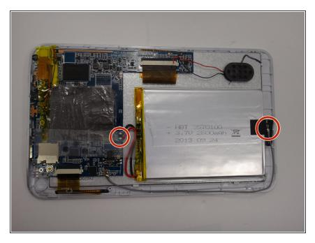
Locate the batteries' connection points.
