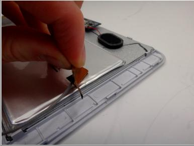
Peel the black sticker off the battery to disconnect the wifi antennae.
