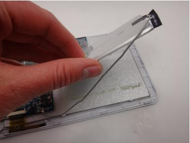
• Remove the old battery and replace it with the new battery.
